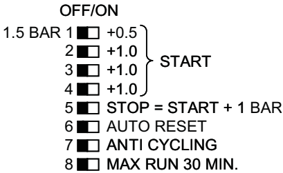
Fig. 6 DIP switches
