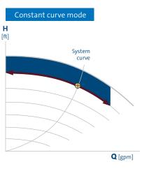
Constant curve mode is used when there is a demand for constant flow and constant head. The pump is adjusted to the desired duty point making pump throttling valves, which are traditionally required in this situation, obsolete.
