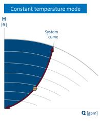
Constant temperature mode is used in variable flow systems within heating, where a constant liquid temperature at a user-defined point, is desired. The pump is in charge of the flow, and external controller for temperature regulation are made unnecessary.
