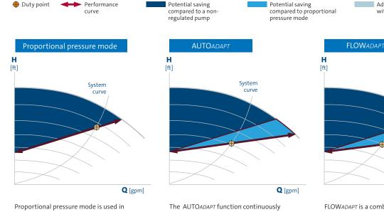
Proportional pressure mode is used in circulating systems. The pump continuously adapts its performance to the varying flow demand.
