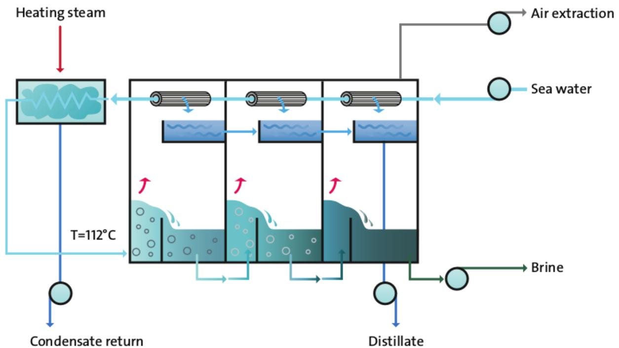
Figure 2 MSF desalination process
