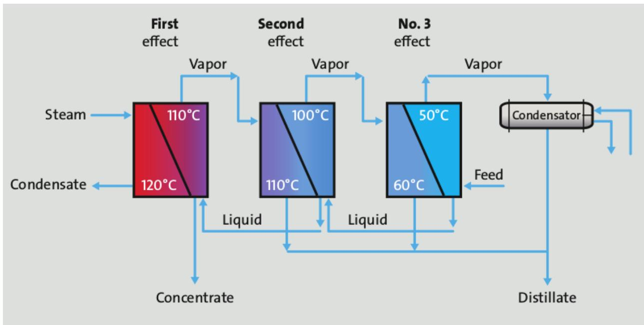
Figure 3 MED desalination process
