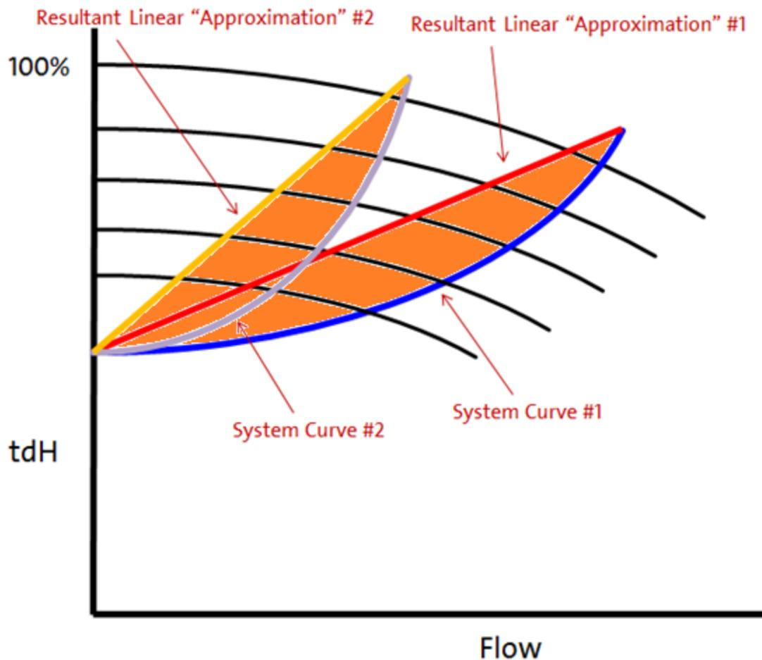
Figure 3 – Linear Approximation for Remote Sensor Simulation
