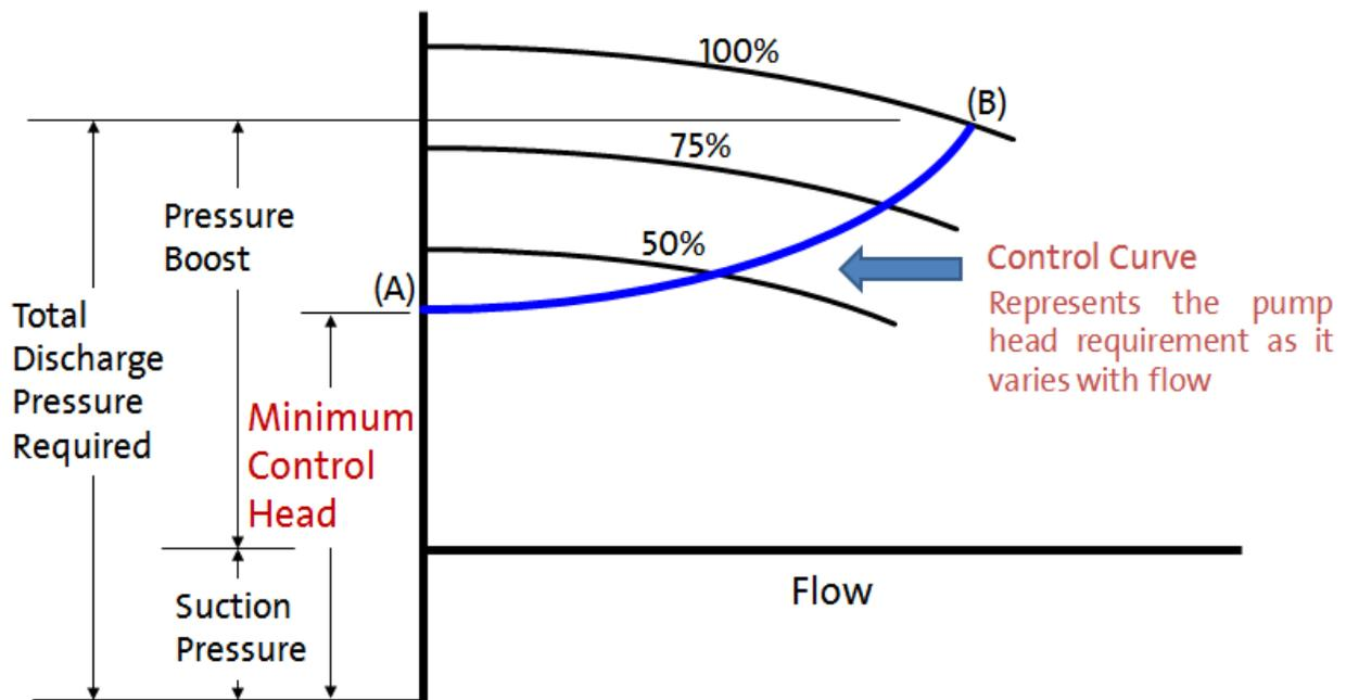
Figure 2 – Proportional Pressure Control Curve
