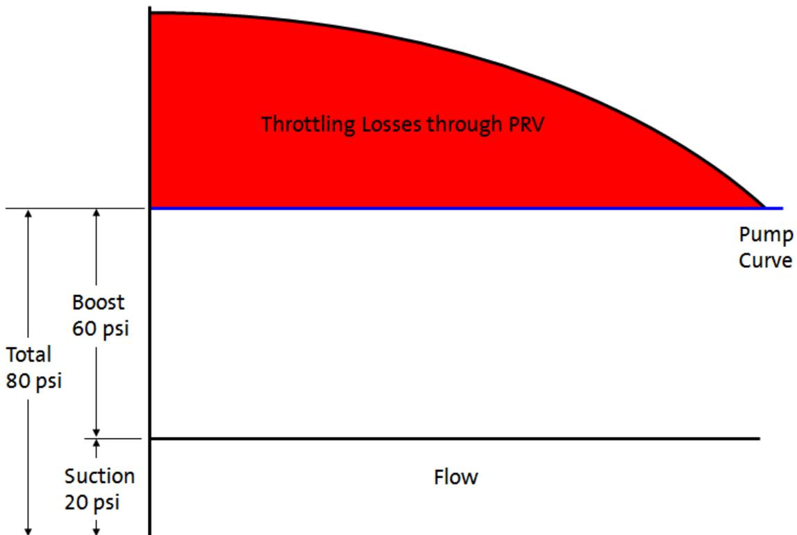
Figure 4 – Constant Speed Pump Pumping Against PRV
