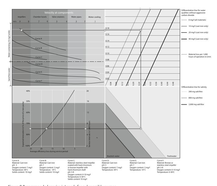
Figure 9 Recommended service intervals for submersible pumps
