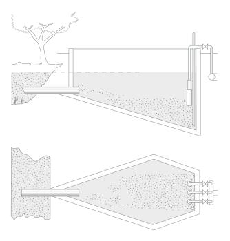
Figure 8 Settling tank principle
