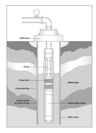
Figure 1 Groundwater well with submersible pump
