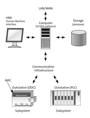
Figure 61 Illustration of the main parts of a SCADA system
