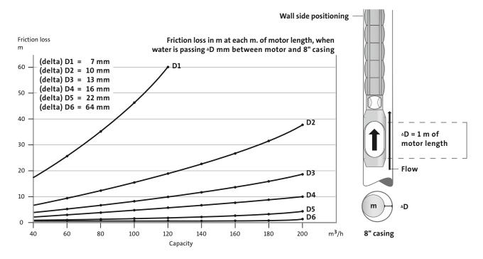
Figure 53 Friction loss, 8"
