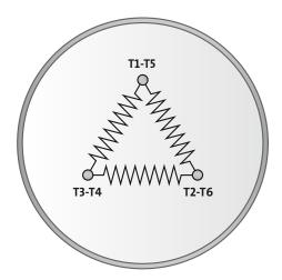
Figure 33. Delta Configuration motor
