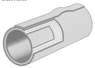
Figure 69 Cross-section of wellmaster hose
