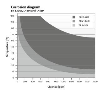
Figure 21 Corrosion diagram
