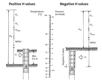
Figure 16 Installation depth
