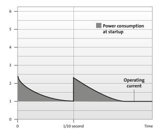
Figure 34 Current flow by autotransformer starting
