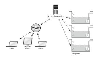
Figure 62 Illustration of the princible in web-hosted SCADA
