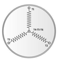
Figure 32. Wye configuration at start-up
