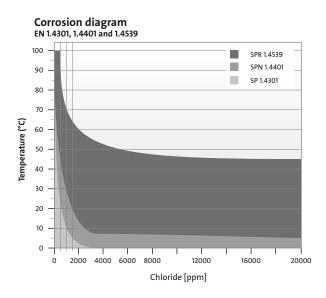
Figure 22 Corrosion diagram
