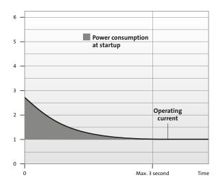
Figure 38 Current flow by soft starting
