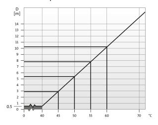
Figure 58 Required water temperature/installation depth of MS 4000 and MS 6000
