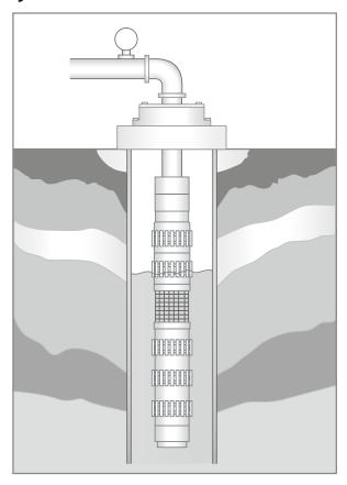
Figure 67 Submersible pump set with sacrificial zinc anodes.
