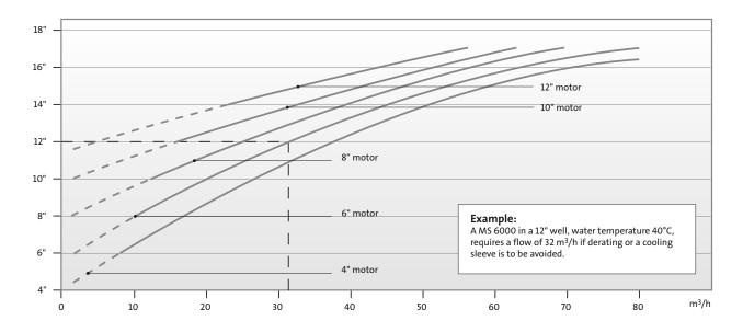
Figure 56 Maximum full-load cooling water temperature
