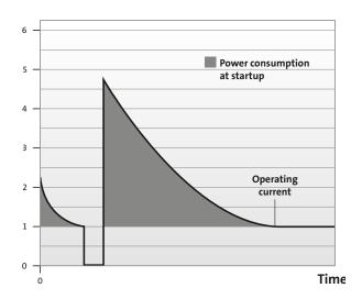
Figure 31 Current flow by SD starting
