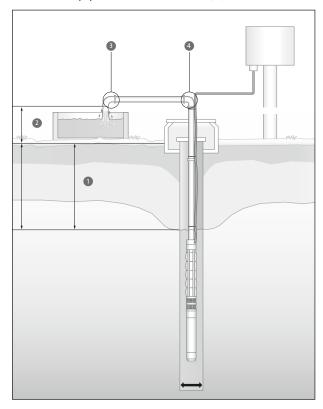
Figure 25 Total head calculation
