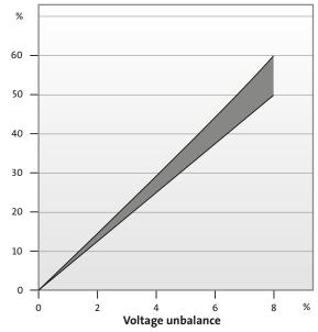
Figure 48 Relationship between voltage and current unbalance
