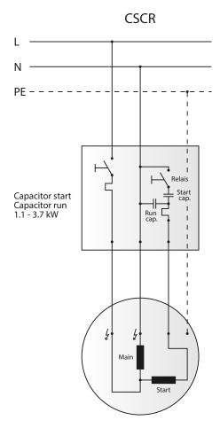
Figure 28 Schematic diagram of a CSCR motor
