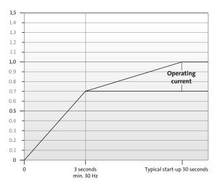
Figure 40 Current flow by frequency converter starting
