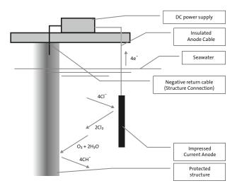
Figure 68 Principle of impressed current cathodic system
