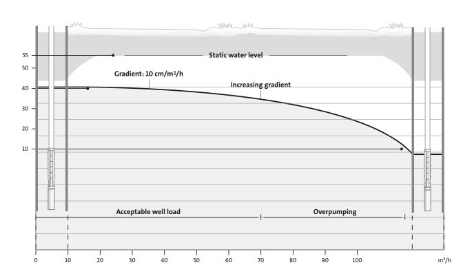
Figure 7 Dynamic water-level variations by test pumping
