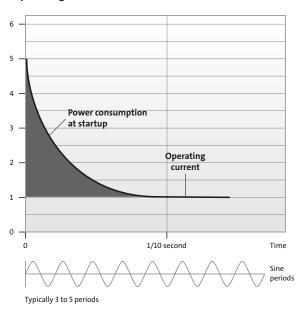
Figure 30 Current flow by DOL starting
