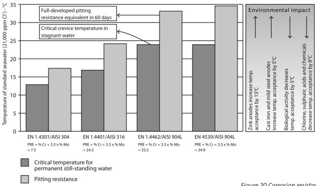
Figure 20 Corrosion resistance
