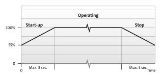
Figure 37 Recommended start-up and stop time, max. 3 sec.
