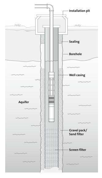
Figure 50 Typical groundwater well components
