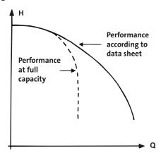
Figure 17 Performance reduction at cavitation
