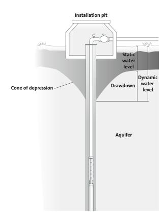
Figure 51 Static and dynamic water level
