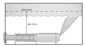
Figure 11 Flow sleeve on horizontally installed pump
