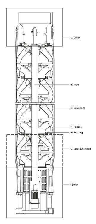
Figure 24 Submersible pump principle
