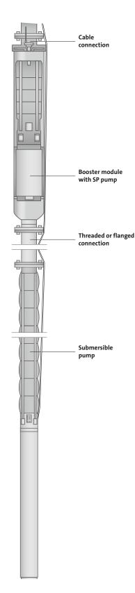
Figure 60 Series coupled submersible pump
