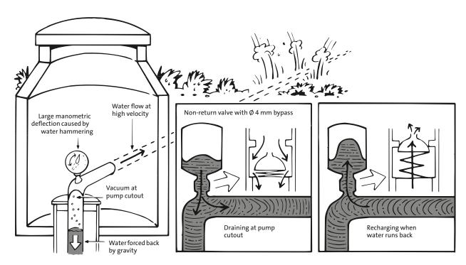
Figure 19 Elimination of water hammer
