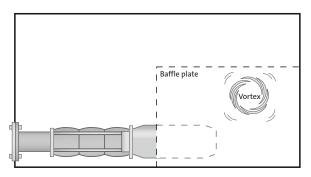
Figure 12 Vortex baffle plate on horizontally-installed pump (seen from above)
