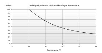
Figure 45 Diagram: Journal bearings load capacity as function of motor liquid temperature.
