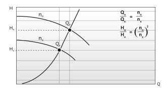
Figure 39 Pump performance with different frequencies
