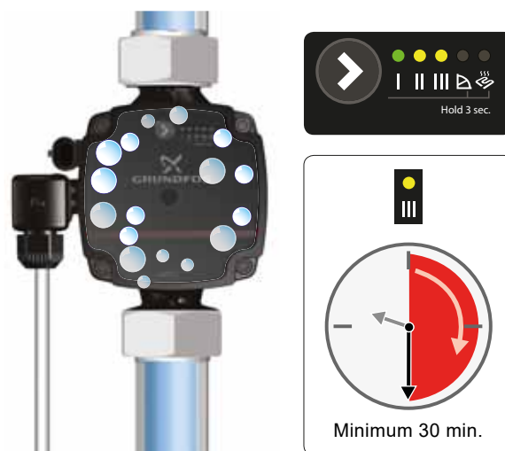
Fig. 7 Venting the pump
